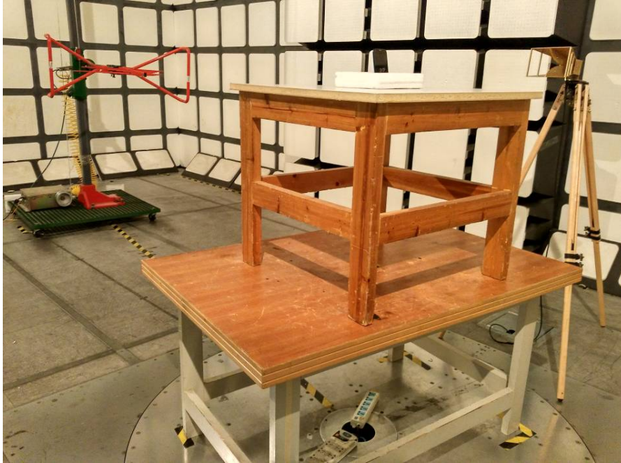
Radiated Emissions Test View (Below 1 GHz)
