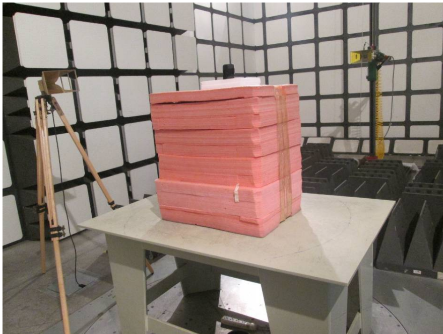
Radiated Emissions Test View (Above 1 GHz)
