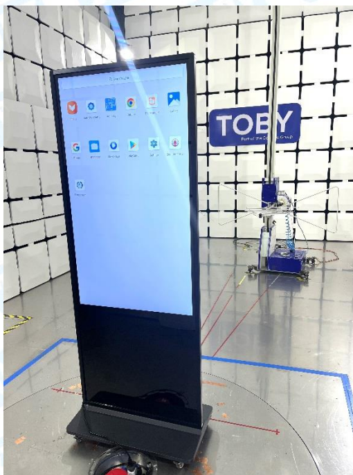
Radiated Emission Test Setup-Below 1G
