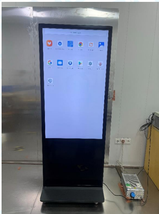
Radiated Emission Test Setup-Below 1G
