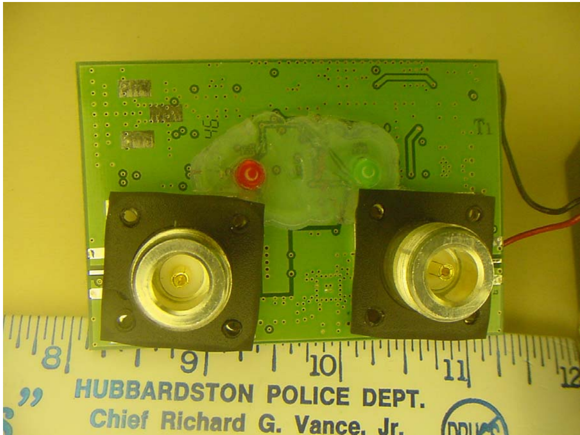
circuit side of amplifier PCB, center is hot glue around the indicator LEDs, gaskets cover the base of the N connectors.
