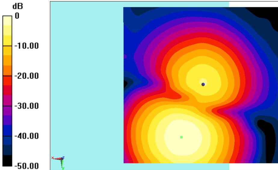
$0 \text{ dB} = 1.258 \text{ A/m} = 1.99 \text{ dBA/m}$ **Fig B.2 T-Coil LTEB12**
