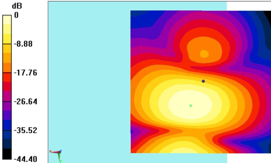
$0 \text{ dB} = 0.7180 \text{ A/m} = -2.88 \text{ dBA/m}$ **Fig B.1 T-Coil LTEB13**
