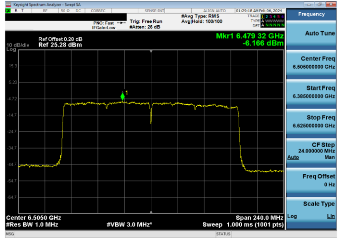
Plot 7-210. Power Spectral Density Plot Antenna WF5B LPI (160MHz 802.11ax (UNII Band 6) – Ch. 111, MCS4)
