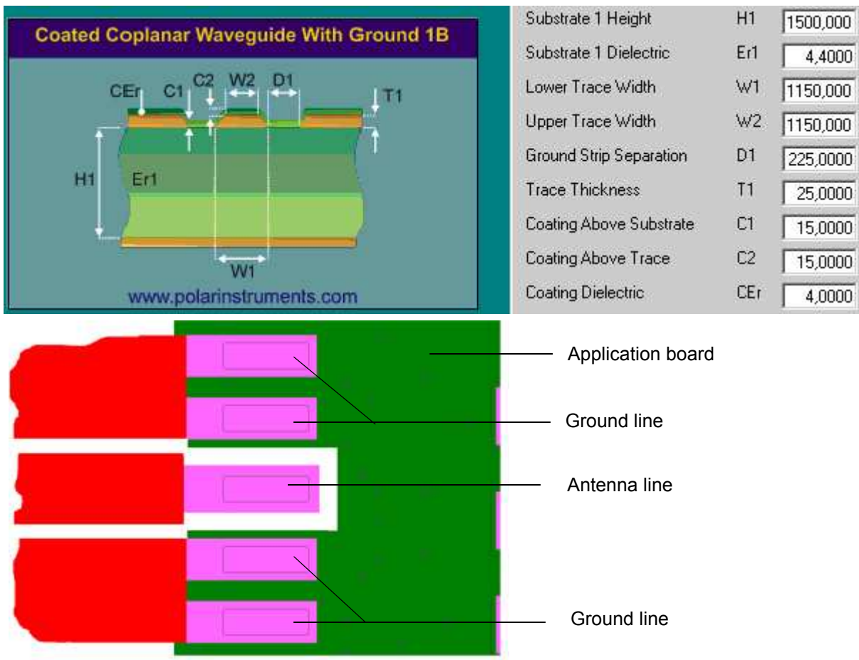
Figure 16: Micro-Stripline on 1.5mm Standard FR4 PCB - example 2
