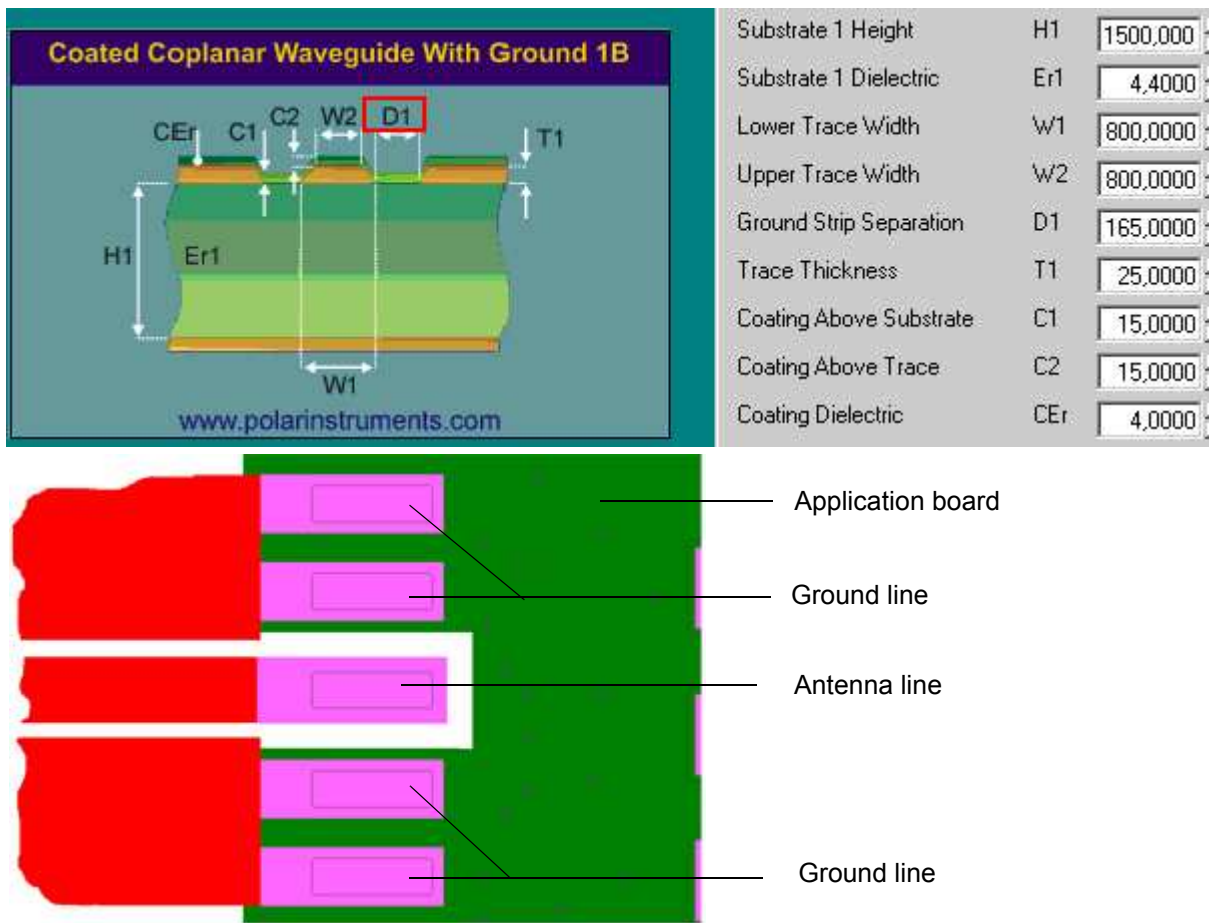
Figure 15: Micro-Stripline on 1.5mm Standard FR4 PCB - example 1
