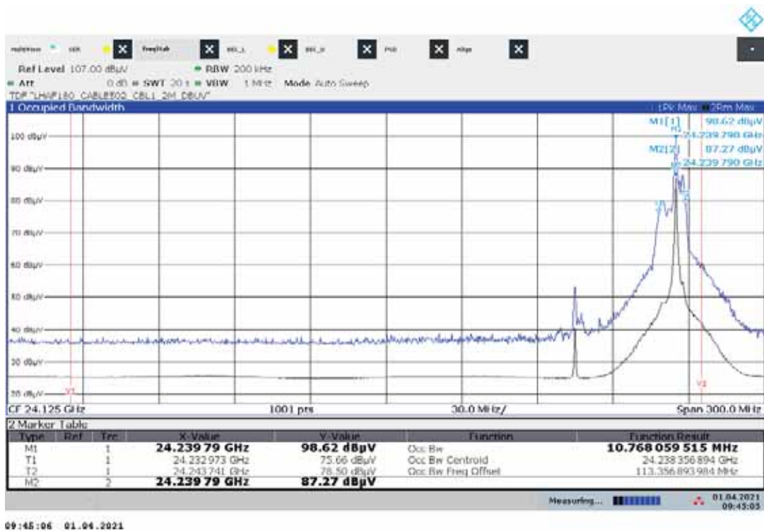
Plot 39: +15 °C, low frequency mode, V_{nom}
