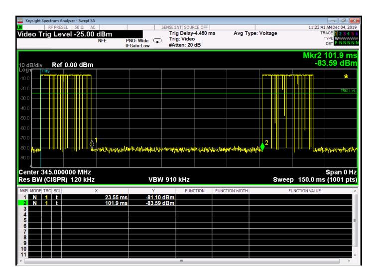
Total On Time in a 100ms Span=23.55ms
