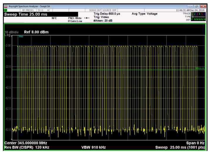
Number of Pulses in Worst Case 100ms=70 Pulse Type 1 On Time=156.4 $\mu$ s\*52=8,132.8 $\mu$ s Pulse Type 2 On Time=297.849 $\mu$ s\*18=5361.28 $\mu$ s 5,361.28 $\mu$ s+8,132.8 $\mu$ s=13.494ms Duty Cycle=13.4941ms/100ms=0.134941 The Peak to Average Duty Cycle Correction= -17.40dB
