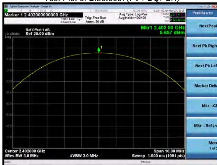
Test Plot of Bluetooth (PI/4-DQPSK)
