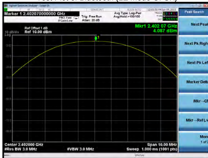
Test Plot of Bluetooth (LE mode GFSK)
