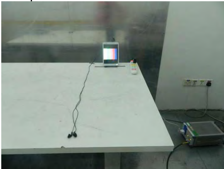
Photograph 2: Set-up for Spurious Emissions
