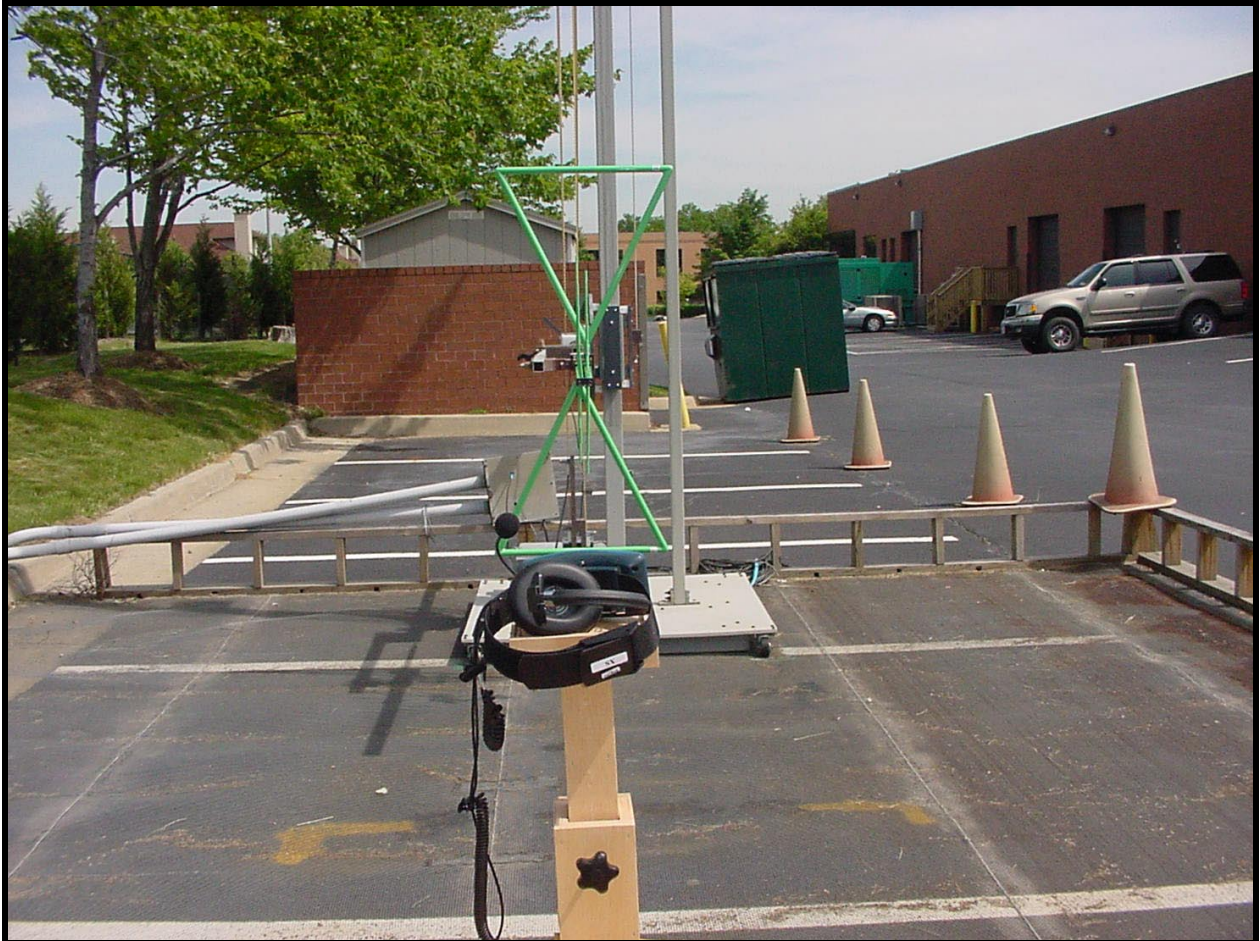
PHOTOGRAPH 3: RADIATED EMISSION REAR VIEW; WORST CASE CONFIGURATION
