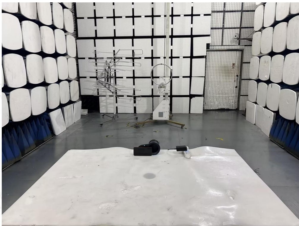
Radiated Emission below 30MHz-AC adapter charge mode
