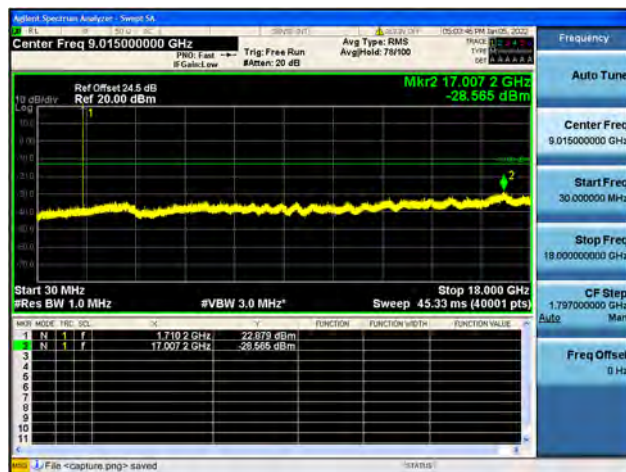
Band66 / 1.4MHz / Mid CH / 16QAM
