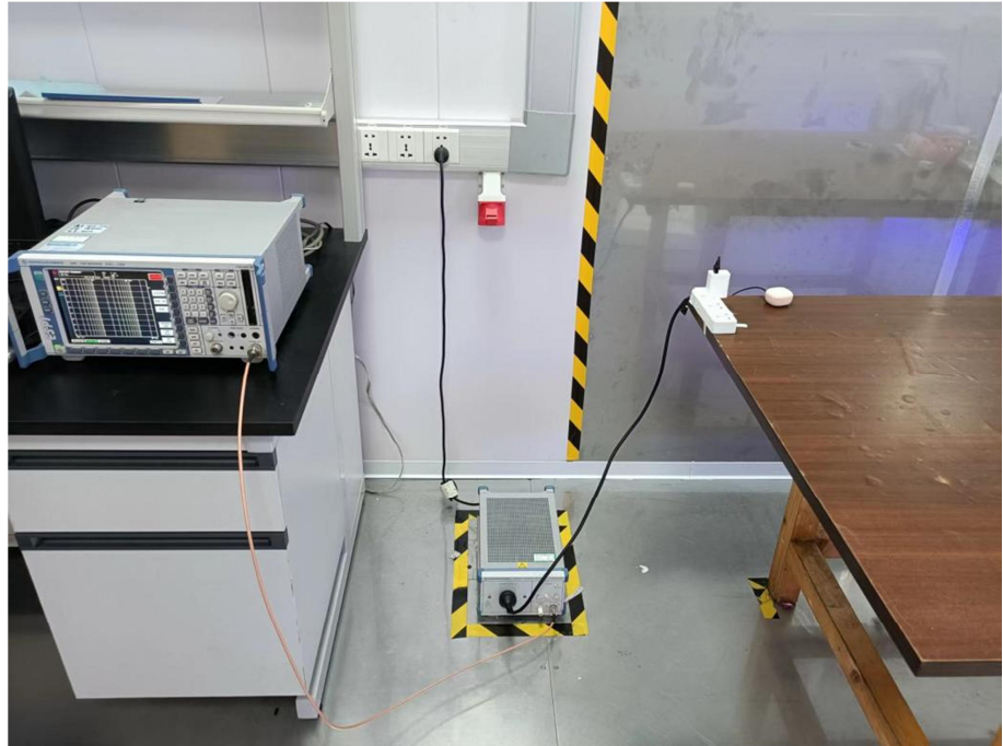
Conducted Emission Test Setup
