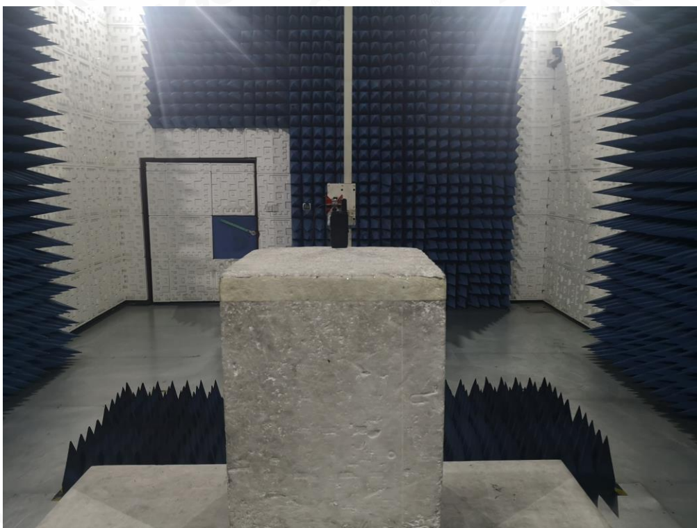
RADIATED EMISSION ABOVE 1G TEST SETUP
