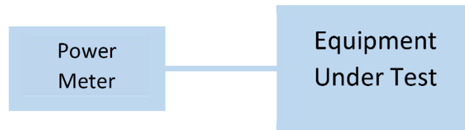
Figure 2: Output Power Measurement
