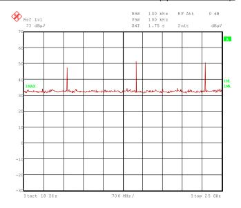
The following frequencies were found inside the restricted bands during the preliminary radiated emission test:
