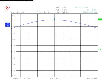
111592 242.wmf: Maximum peak output power at the middle of the assigned frequency band (operation mode 2):
