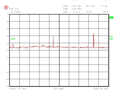
111592 40.wmf: Spurious emissions from 18 GHz to 25 GHz (operation mode 2):
