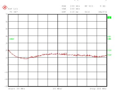
111592 32.wmf: Spurious emissions from 230 MHz to 1 GHz (operation mode 2):
