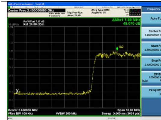
\pi/4 DQPSK(with hopping) Band Edge(CH.0)
