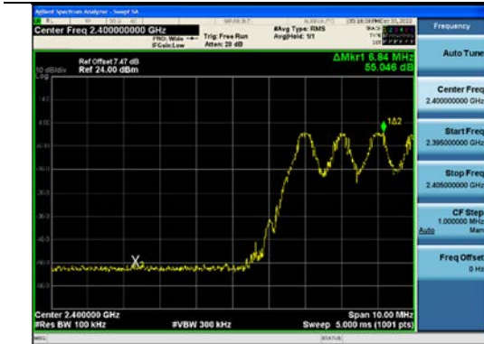
8DPSK(with hopping) Band Edge(CH.0)
