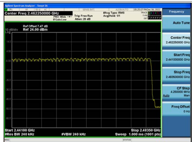
\pi/4 DQPSK Number of Channels (2.441 GHz - 2.483.5 GHz)
