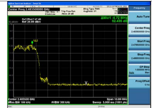
\pi/4 DQPSK (with hopping) Band Edge(CH.78)
