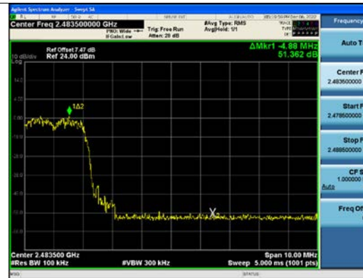
\pi/4 DQPSK (with hopping) Band Edge(CH.78)
