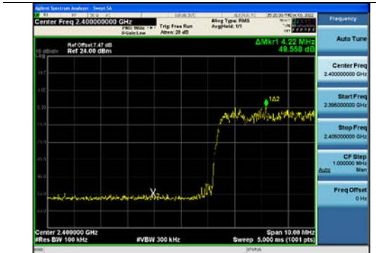
\pi/4 DQPSK(with hopping) Band Edge(CH.0)
