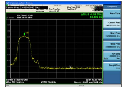
\pi/4 DQPSK (without hopping) Band Edge(CH.78)
