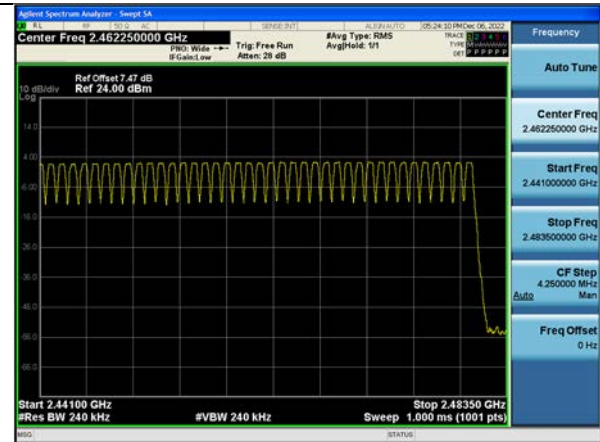
8DPSK Number of Channels (2.441 GHz - 2.483.5 GHz)
