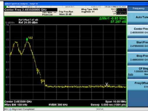
8DPSK(with hopping) Band Edge(CH.78)
