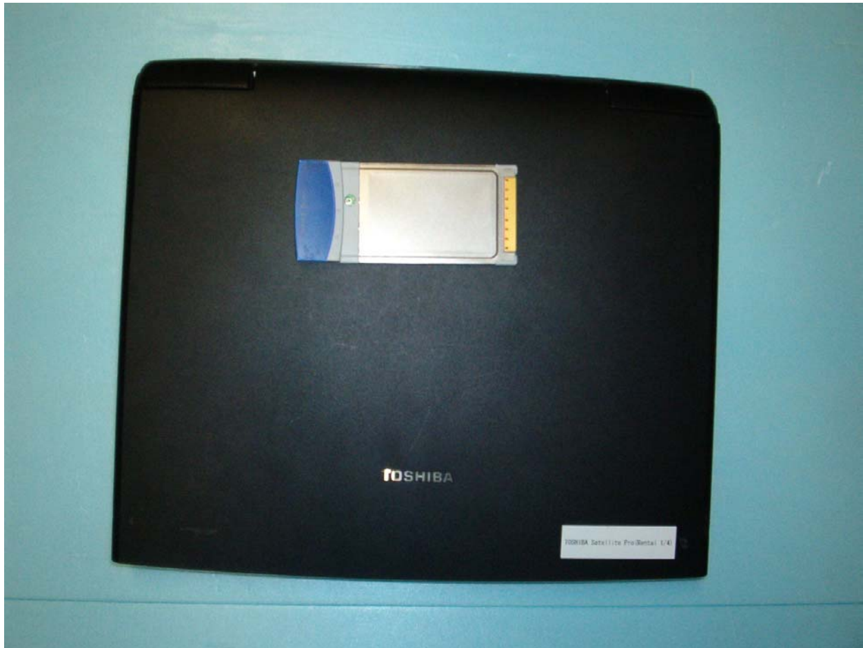
Fig. 2. A picture of the Askey Corporation 802.11 a/b Cardbus Card placed on the Toshiba laptop computer.
