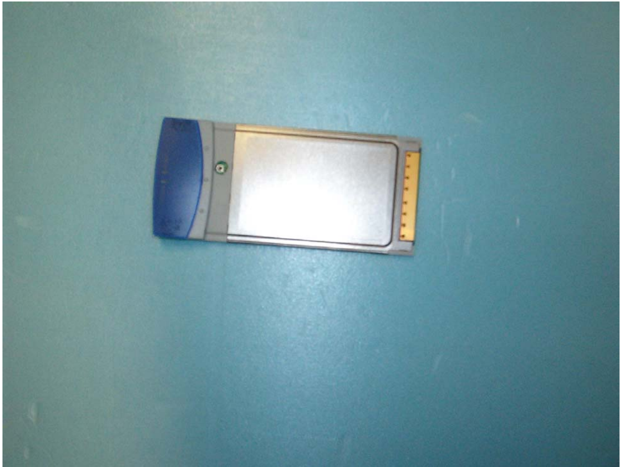
Fig. 12. Photograph of the Askey Corporation 802.11 a/b Cardbus Card with coaxial output for conducted power measurements.
