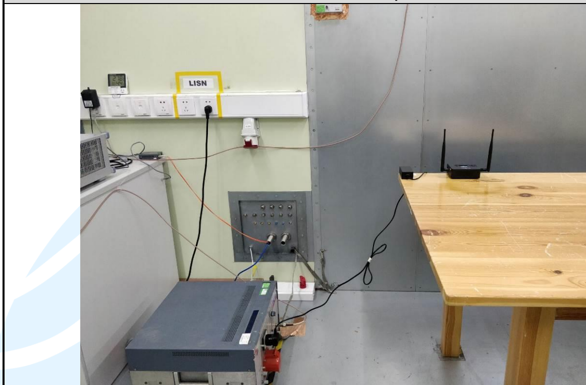
Conducted Emission Test Setup-3 - Mode 4
