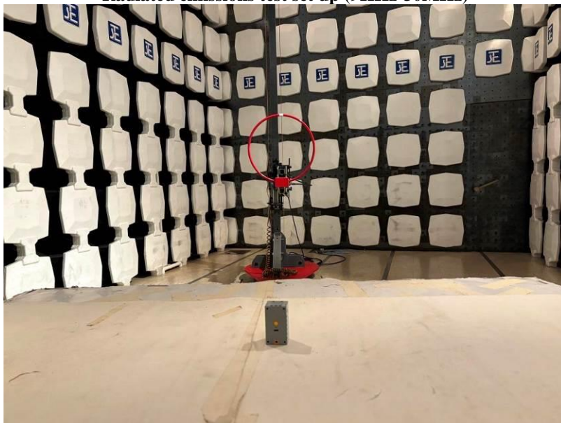
Radiated emissions test set up (9KHz-30MHz)
