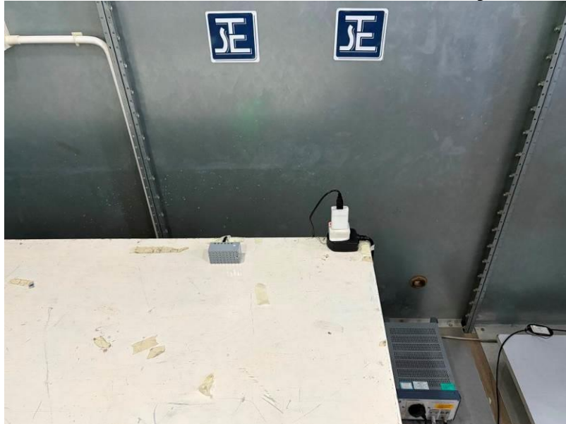
Measurement of Conducted Emission Test Set Up
