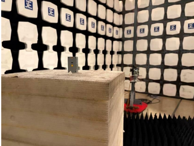
Radiated emissions test set up (Above 1GHz)
