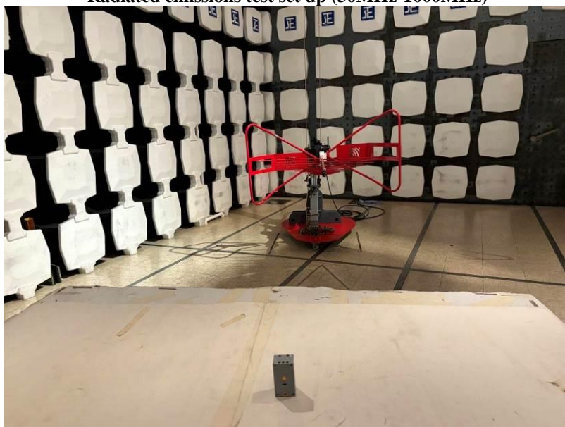
Radiated emissions test set up (30MHz-1000MHz)
