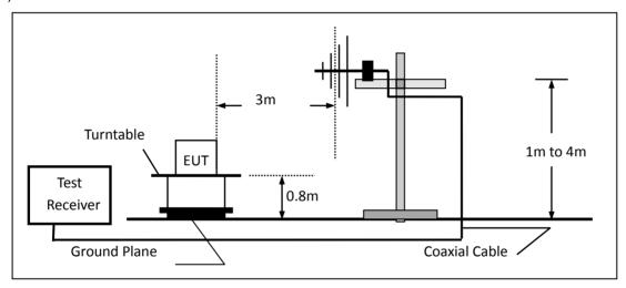
(c) For radiated emissions above 1000MHz
