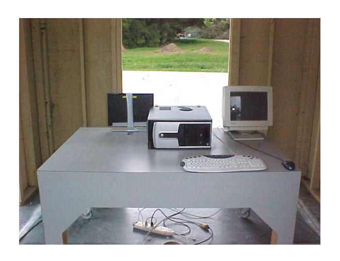
Radiated Emissions Measurement (Front View) Setup
