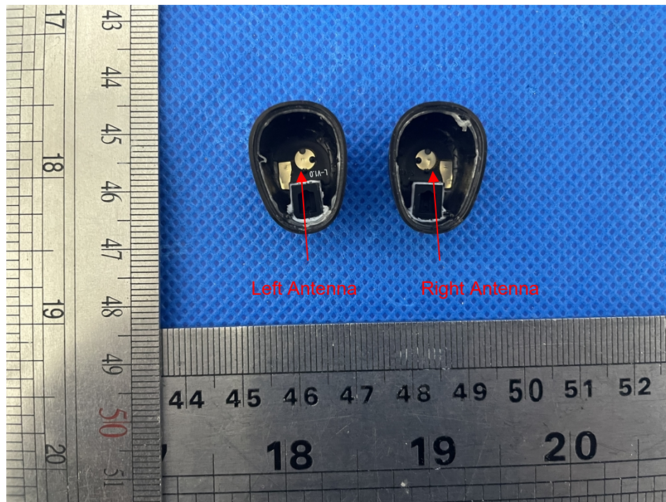
Figure 11 Antenna view of Left & ear buds
