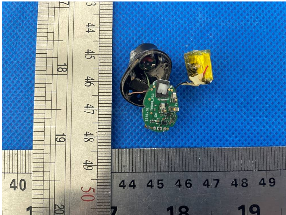
Figure 9 PCB view 2 of R ear bud
