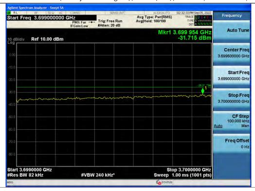
+3 dB above Out-of-band (two adjacent test signals) / C-Band(Ant2) / Downlink / 5G NR 80 MHz / Upper
