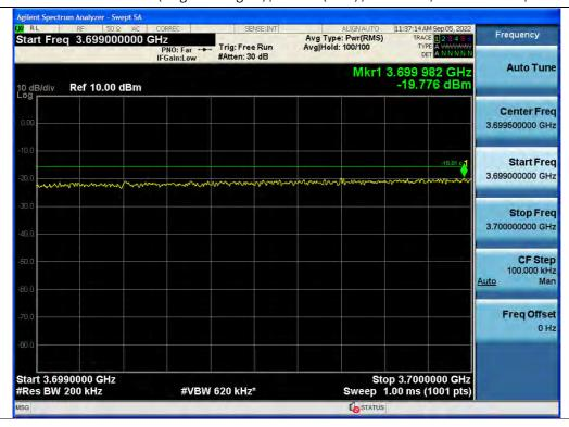
+3 dB above Out-of-band (single test signal) / C-Band(Ant1) / Downlink / 5G NR 20 MHz / Upper
