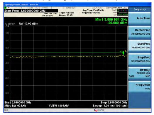
+3 dB above Out-of-band (single test signal) / C-Band(Ant1) / Downlink / 5G NR 60 MHz / Upper
