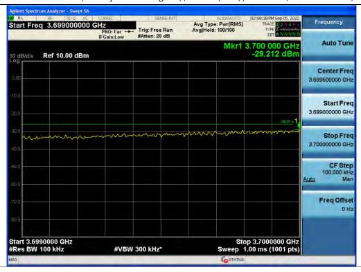
+3 dB above Out-of-band (two adjacent test signals) / C-Band(Ant2) / Downlink / 5G NR 100 MHz / Upper
