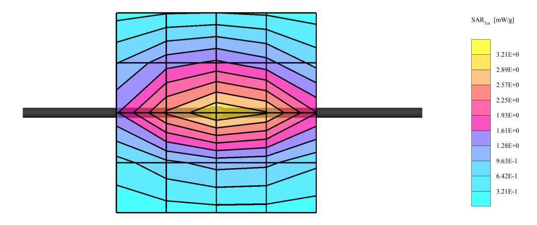
SAM 1 (Cellular - Brain Tissue) Frequency: 900 MHz; Crest factor: 1.0 Validation 900MHz - Brain Tissue:  $\sigma = 0.99$  mho/m  $\varepsilon_r = 41.0 \ \rho = 1.00 \ g/cm^3$ Probe: ET3DV6 - SN1504; ConvF(6.50,6.50,6.50) Cubes (2): Peak: 4.80 mW/g ± 0.05 dB, SAR (1g): 2.96 mW/g ± 0.06 dB, SAR (10g): 1.85 mW/g ± 0.06 dB, (Worst-case extrapolation) Penetration depth: 11.2 (10.1, 12.7) [mm] Powerdrift: -0.17 dB Liquid Temperature (°C): 20.6
