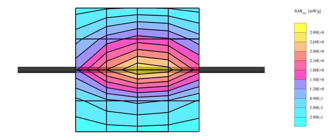
SAM 1 (Cellular - Brain Tissue) Frequency: 900 MHz; Crest factor: 1.0 Validation 900MHz - Brain Tissue:  $\sigma = 1.00$  mho/m  $\varepsilon_r = 39.6 \ \rho = 1.00$  g/cm<sup>3</sup> Probe: ET3DV6 - SN1504; ConvF(6.50,6.50,6.50) Cubes (2): Peak: 4.32 mW/g ± 0.07 dB, SAR (1g): 2.65 mW/g ± 0.06 dB, SAR (10g): 1.65 mW/g ± 0.06 dB, (Worst-case extrapolation) Penetration depth: 11.0 (10.0, 12.4) [mm] Powerdrift: -0.04 dB Liquid Temperature (°C): 20.5
