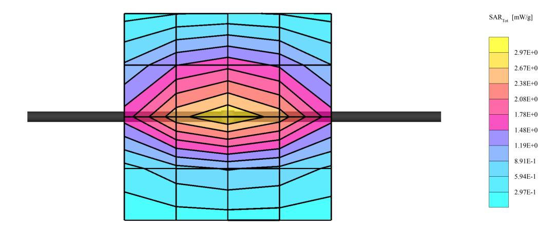
SAM 1 (Cellular - Brain Tissue) Frequency: 900 MHz; Crest factor: 1.0 Validation 900MHz - Brain Tissue:  $\sigma = 0.98$  mho/m  $\varepsilon_r = 40.2 \ \rho = 1.00 \ g/cm^3$ Probe: ET3DV6 - SN1504; ConvF(6.50,6.50,6.50) Cubes (2): Peak: 4.83 mW/g  $\pm 0.06$  dB, SAR (1g): 2.97 mW/g  $\pm 0.05$  dB, SAR (10g): 1.86 mW/g  $\pm 0.05$  dB, (Worst-case extrapolation) Penetration depth: 11.2 (10.1, 12.7) [mm] Powerdrift: -0.15 dB Liquid Temperature (°C): 20.0
