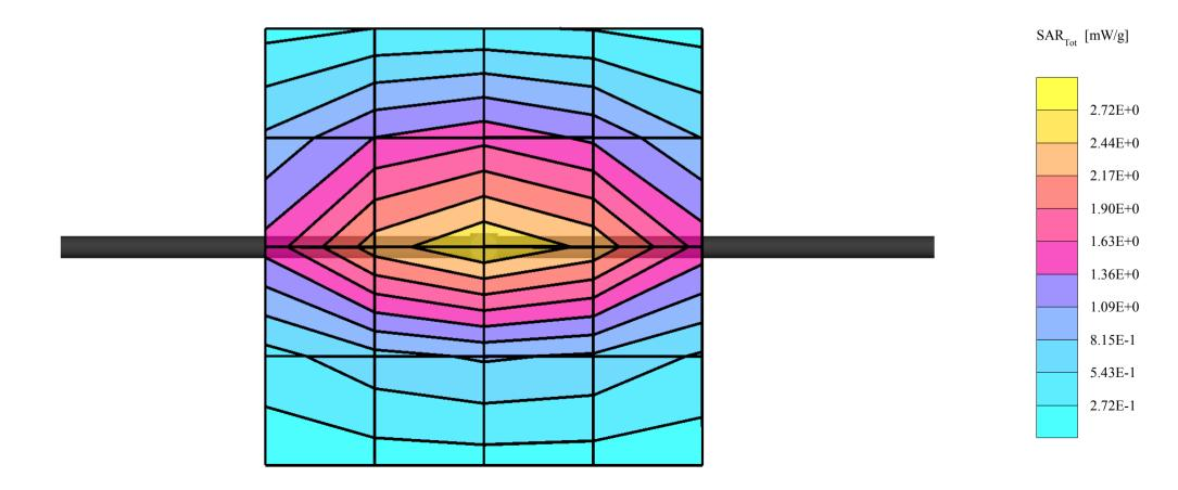
SAM 1 (Cellular - Brain Tissue) Frequency: 900 MHz; Crest factor: 1.0 Validation 900MHz - Brain Tissue:  $\sigma = 1.02$  mho/m  $\varepsilon_r = 39.5 \rho = 1.00$  g/cm<sup>3</sup> Probe: ET3DV6 - SN1504; ConvF(6.50,6.50,6.50) Cubes (2): Peak: 5.09 mW/g ± 0.08 dB, SAR (1g): 3.11 mW/g ± 0.07 dB, SAR (10g): 1.94 mW/g ± 0.07 dB, (Worst-case extrapolation) Penetration depth: 11.0 (9.9, 12.5) [mm] Powerdrift: -0.12 dB Liquid Temperature (°C): 20.3
