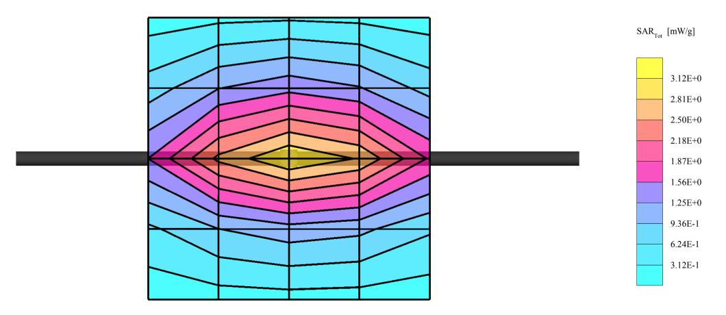
SAM 1 (Cellular - Brain Tissue) Frequency: 900 MHz; Crest factor: 1.0 Validation 900MHz - Brain Tissue:  $\sigma = 0.97$  mho/m  $\varepsilon_r = 39.5 \ \rho = 1.00 \ g/cm^3$ Probe: ET3DV6 - SN1504; ConvF(6.50,6.50,6.50) Cubes (2): Peak: 4.73 mW/g ± 0.07 dB, SAR (1g): 2.93 mW/g ± 0.07 dB, SAR (10g): 1.83 mW/g ± 0.06 dB, (Worst-case extrapolation) Penetration depth: 11.2 (10.2, 12.7) [mm] Powerdrift: -0.19 dB Liquid Temperature (°C): 20.2
