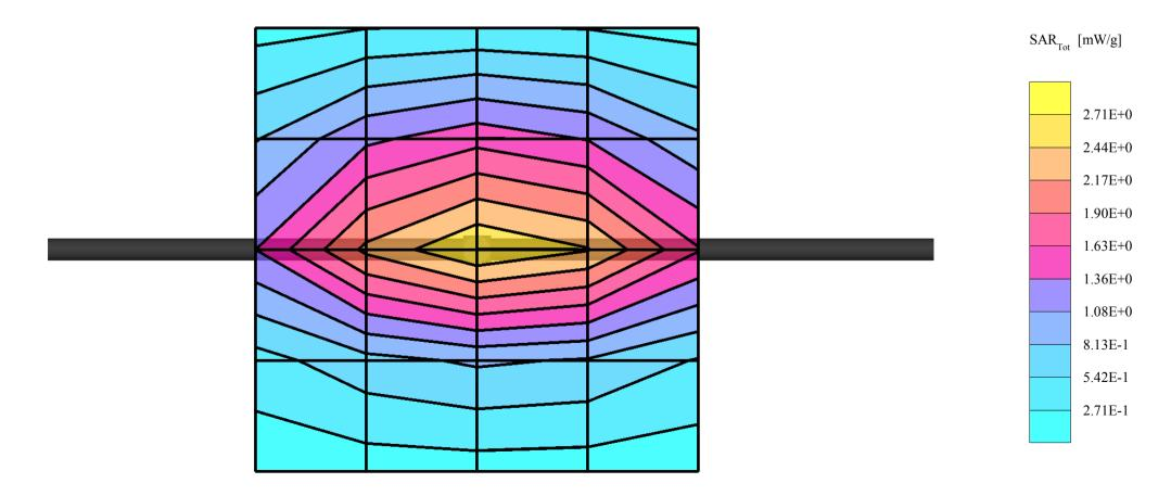
SAM 1 (Cellular - Brain Tissue) Frequency: 900 MHz; Crest factor: 1.0 Validation 900MHz - Brain Tissue:  $\sigma = 0.99$  mho/m  $\varepsilon_r = 39.7 \ \rho = 1.00 \ g/cm^3$ Probe: ET3DV6 - SN1504; ConvF(6.50,6.50,6.50) Cubes (2): Peak: 4.85 mW/g ± 0.06 dB, SAR (1g): 2.96 mW/g ± 0.06 dB, SAR (10g): 1.84 mW/g ± 0.06 dB, (Worst-case extrapolation) Penetration depth: 10.9 (9.9, 12.3) [mm] Powerdrift: -0.05 dB Liquid Temperature (°C): 20.3
