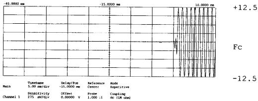
Trigger mode : Edge On Positive Edge Of Chan2 Trigger Level Chan2 - -962.500 mV (noise reject ON) Holdoff - 40.000 ns
