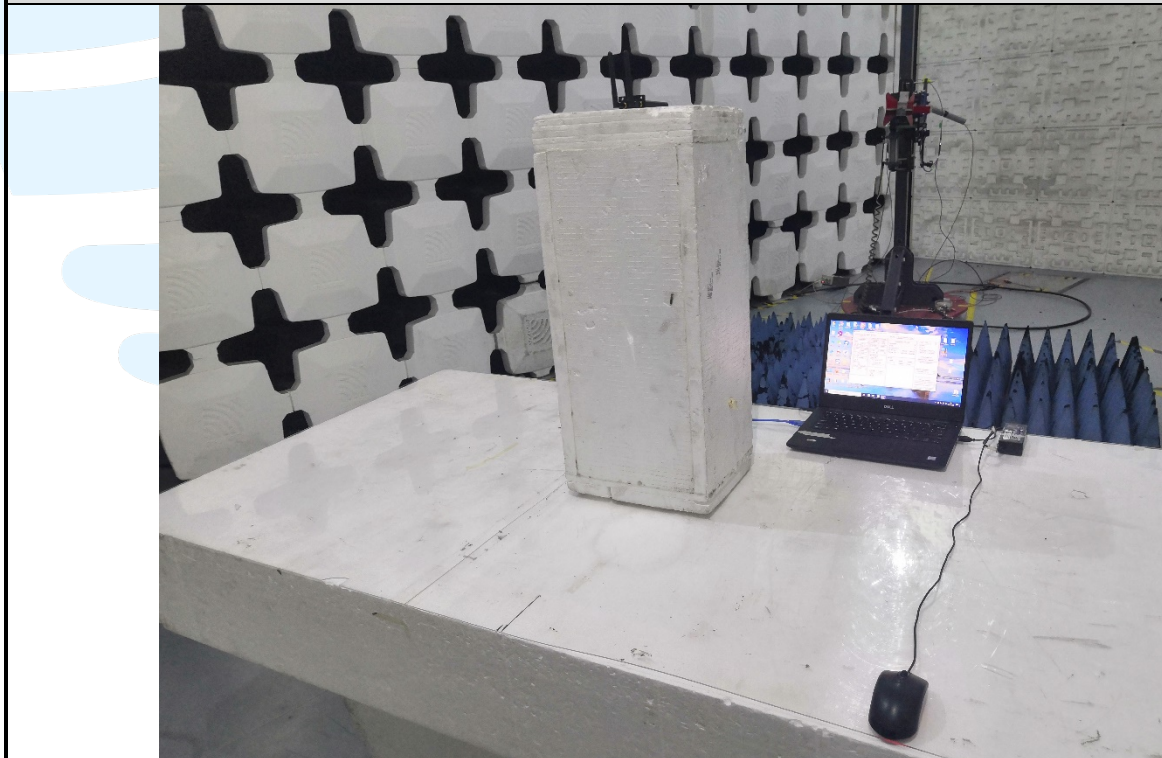
Radiated emission Test Setup (Above 1 GHz)
