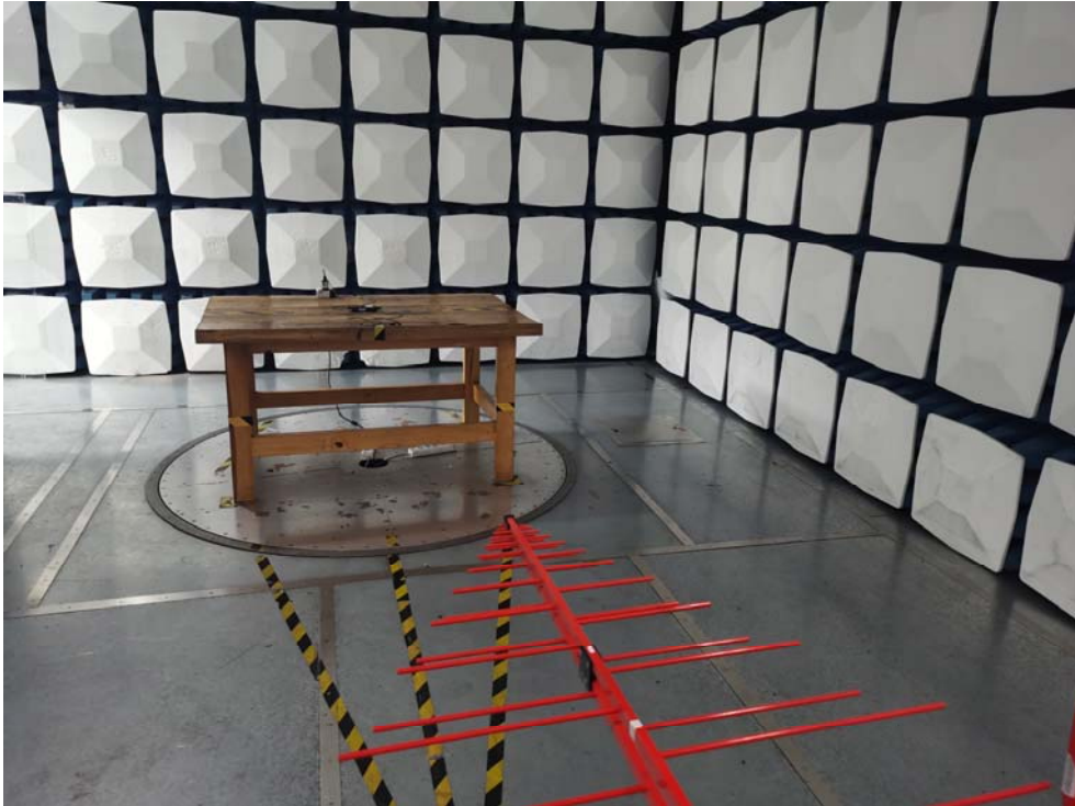
Radiated Emission Above 1GHz View
