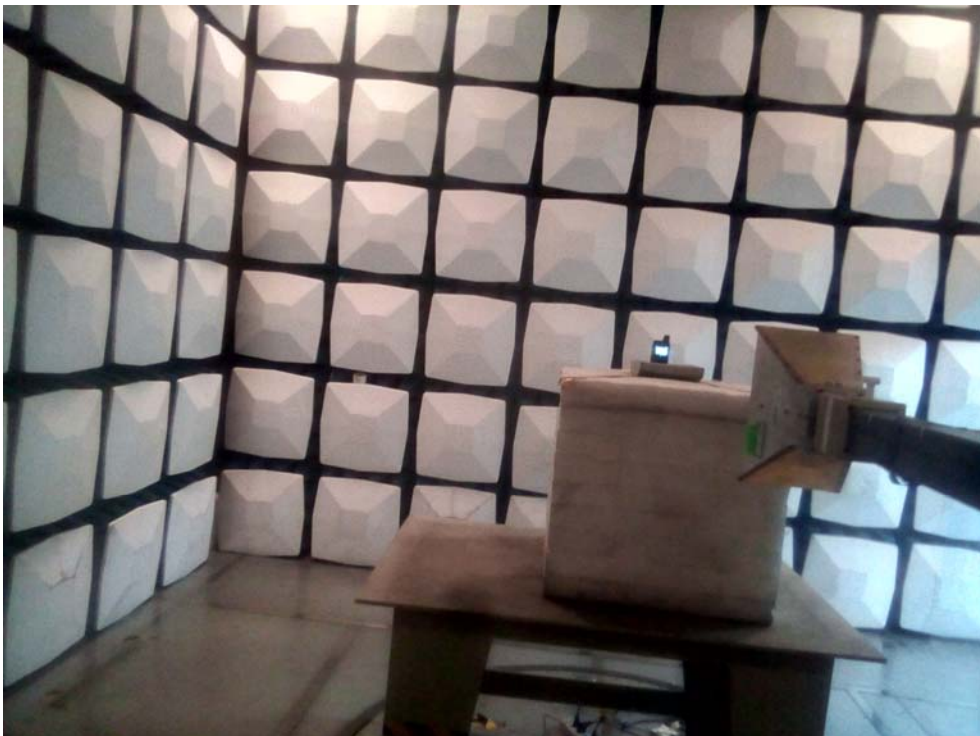
Radiated Emission Above 1GHz View
