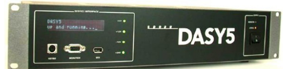
Picture C.8 Server for DASY 5
