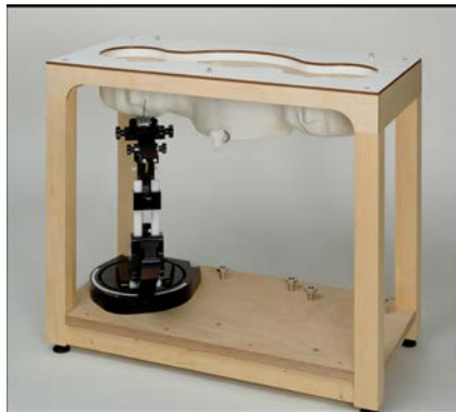
Picture C.10: SAM Twin Phantom
