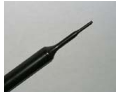
Picture C.2 Near-field Probe
