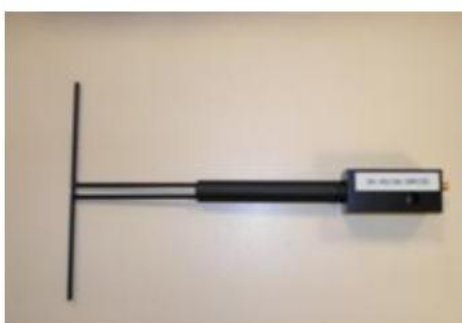
Figure 1 – Satimo COMOSAR Validation Dipole
