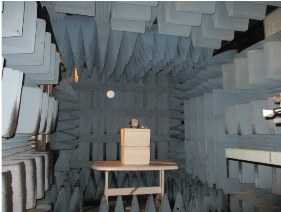
Figure 4. Radiated Emission Test, 26.5-40.0GHz
