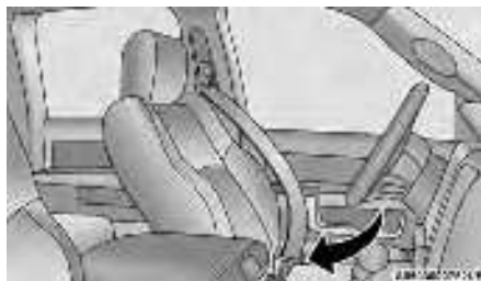
Inserting Latch Plate Into Buckle
