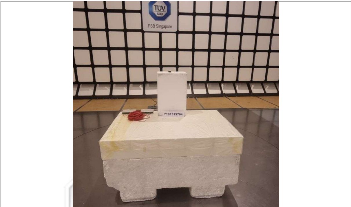
Spectrum Bandwidth (20dB Bandwidth Measurement)
