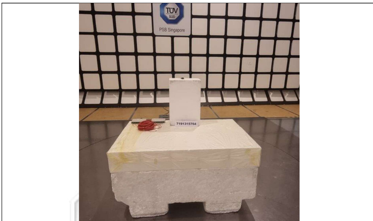
Radiated Emissions (Spurious Emissions Inclusive Restricted Bands Requirement) Test Setup (Front View)
