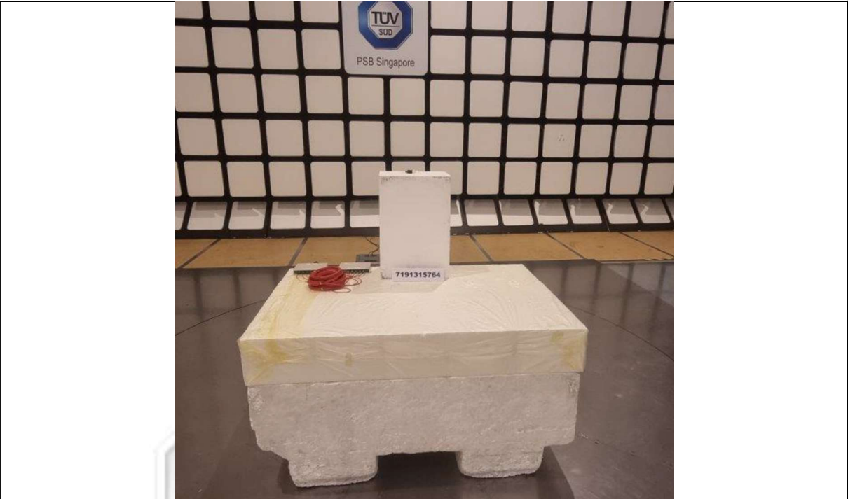
Radiated Emissions (Fundamental) Test Setup (Front View)
