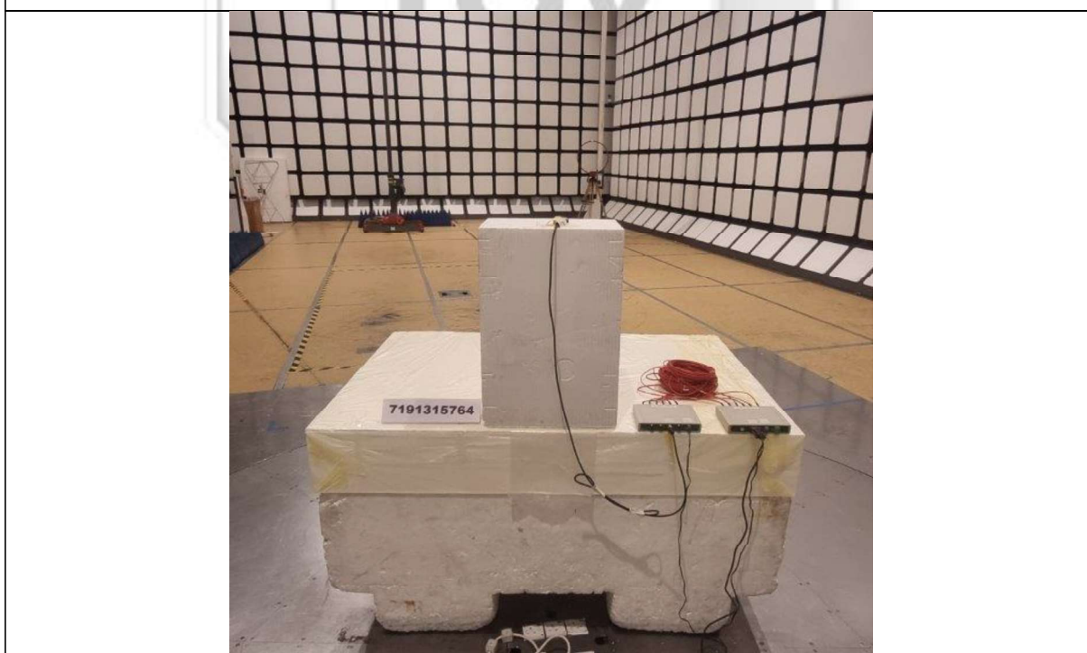
Radiated Emissions (Spurious Emissions Inclusive Restricted Bands Requirement) Test Setup (Rear View)
