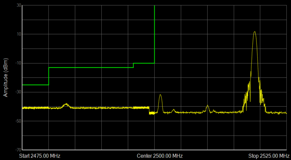
Band7 QPSK BW=20MHz Channel=20850 RB Size=1 Position=#Max
