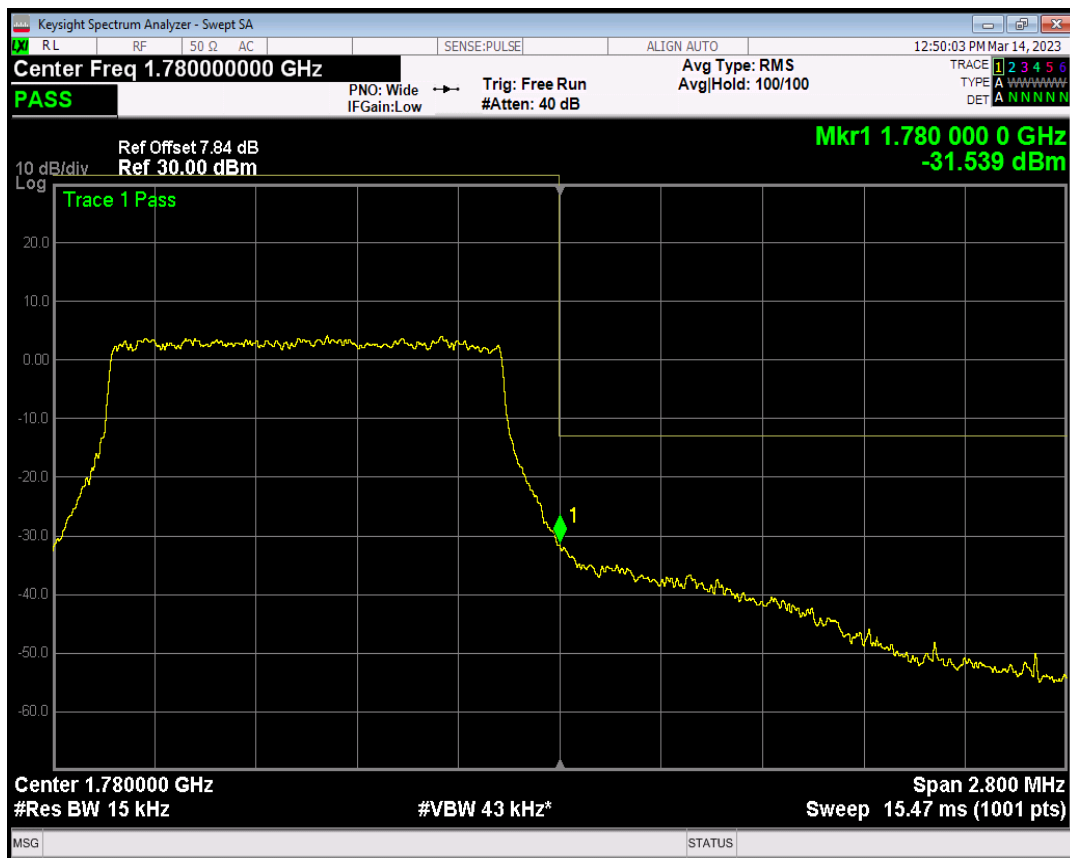
Band66 QPSK BW=3MHz Channel=131987 RB Size=1 Position=#0
