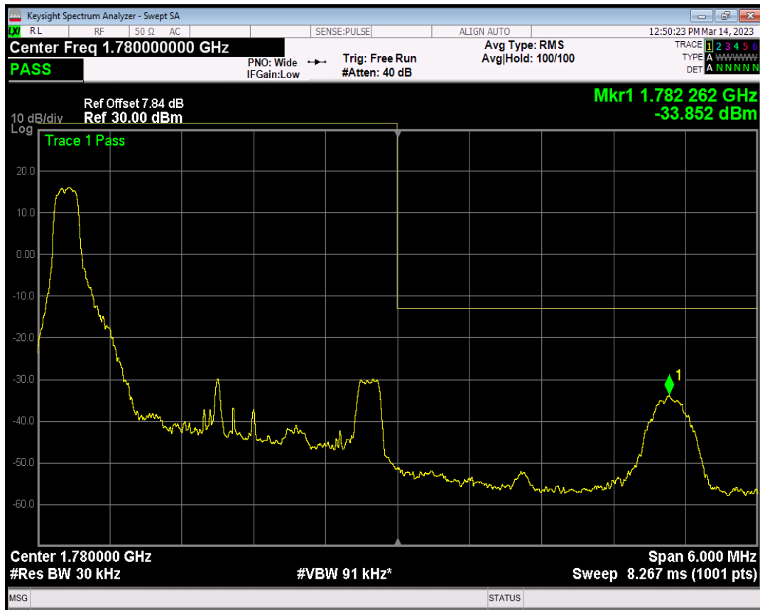
Band66 QPSK BW=3MHz Channel=132657 RB Size=1 Position=#Max
