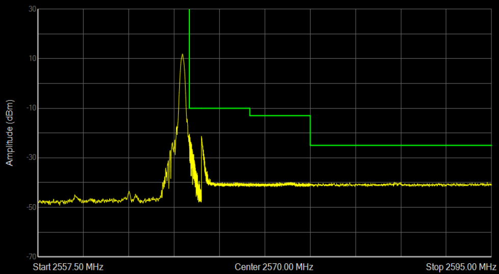
Band7 QPSK BW=10MHz Channel=21400 RB Size=1 Position=#Max
