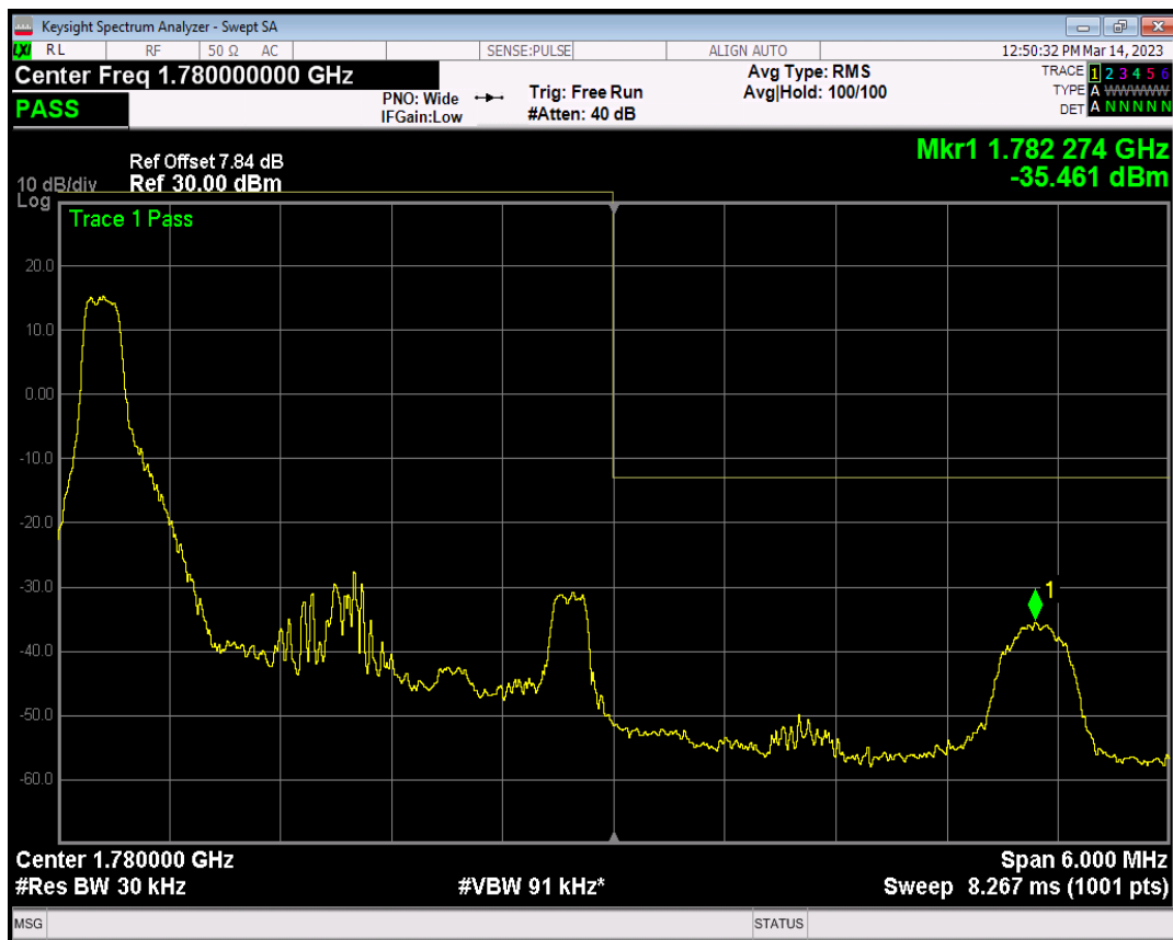
Band66 QAM16 BW=3MHz Channel=132657 RB Size=1 Position=#Max
