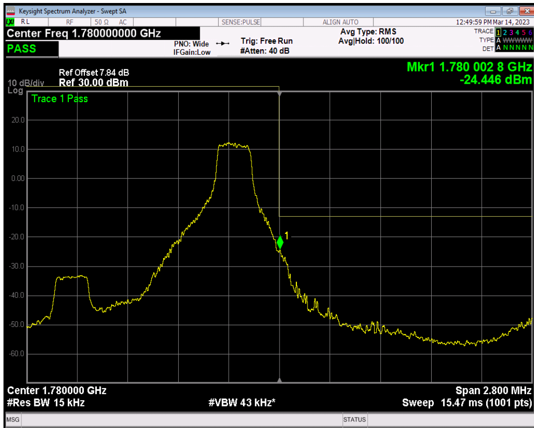
Band66 QAM16 BW=1.4MHz Channel=132665 RB Size=6 Position=#0
