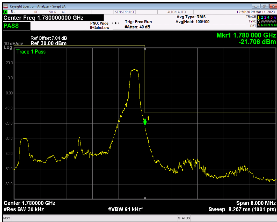
Band66 QPSK BW=3MHz Channel=132657 RB Size=15 Position=#0
