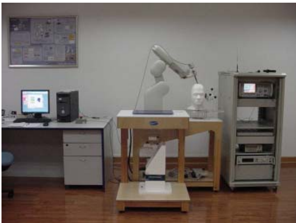
Fig.1 SARA2 System Test Layout
