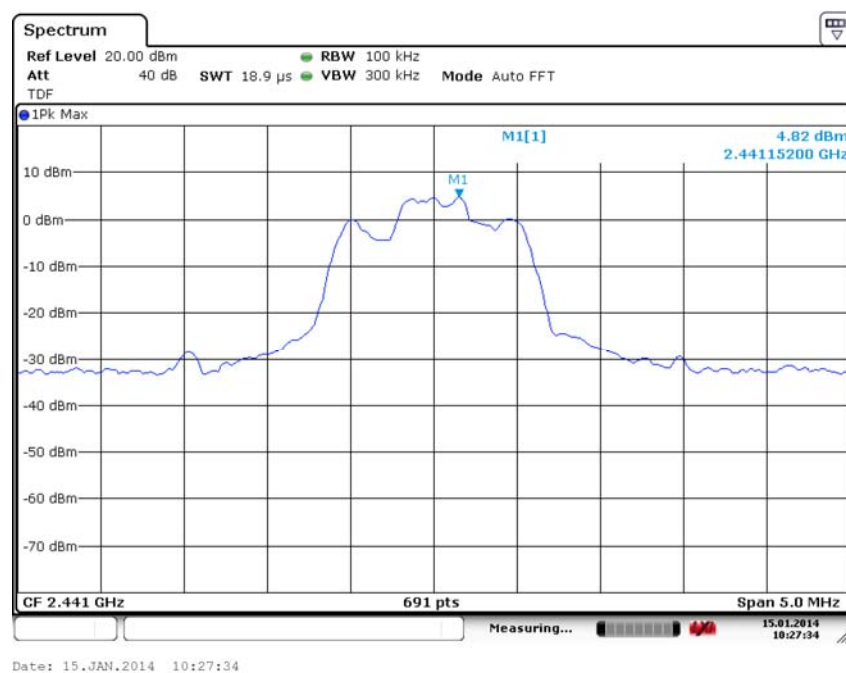
Fig. 25 Conducted Spurious Emission ( \pi/4 DQPSK, Ch39, 2.441GHz)
