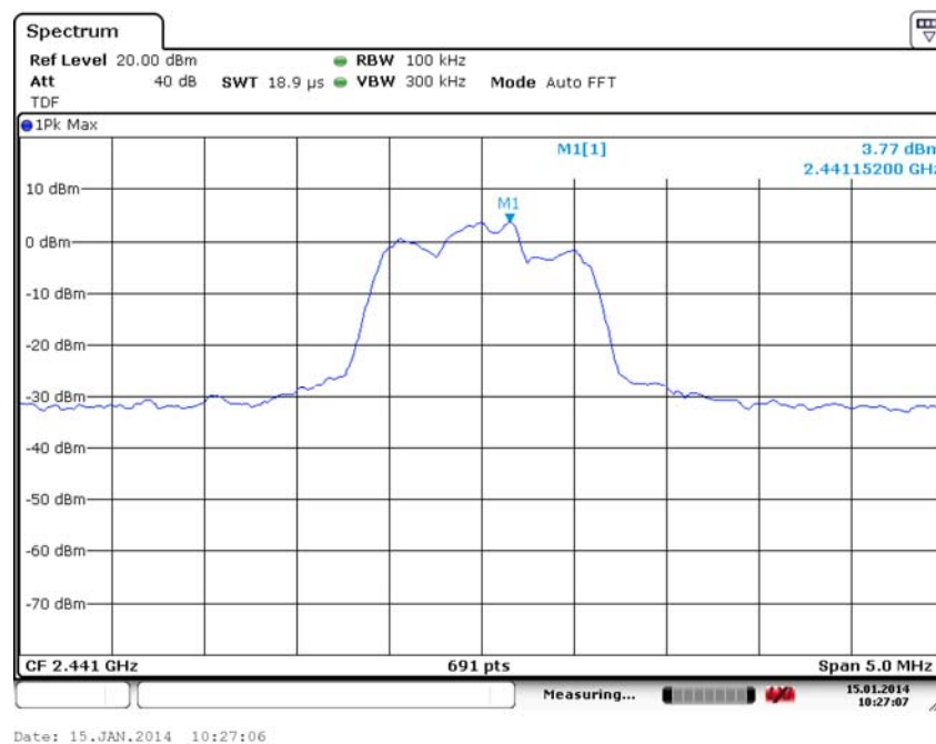
Fig. 34 Conducted Spurious Emission (8DPSK, Ch39, 2.441GHz)
