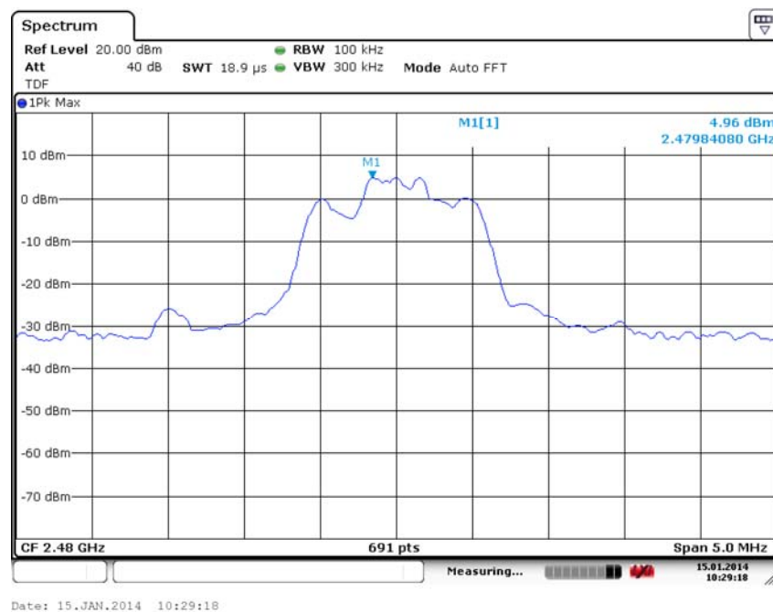
Fig. 28 Conducted Spurious Emission ( \pi/4 DQPSK, Ch78, 2.480GHz)
