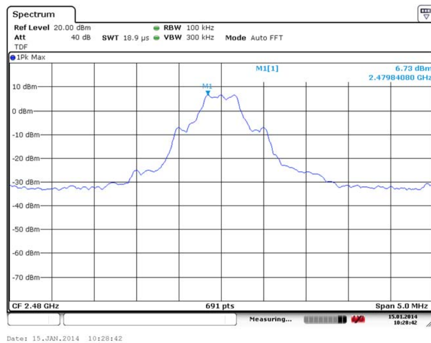
Fig. 19 Conducted Spurious Emission (GFSK, Ch78, 2.480GHz)
