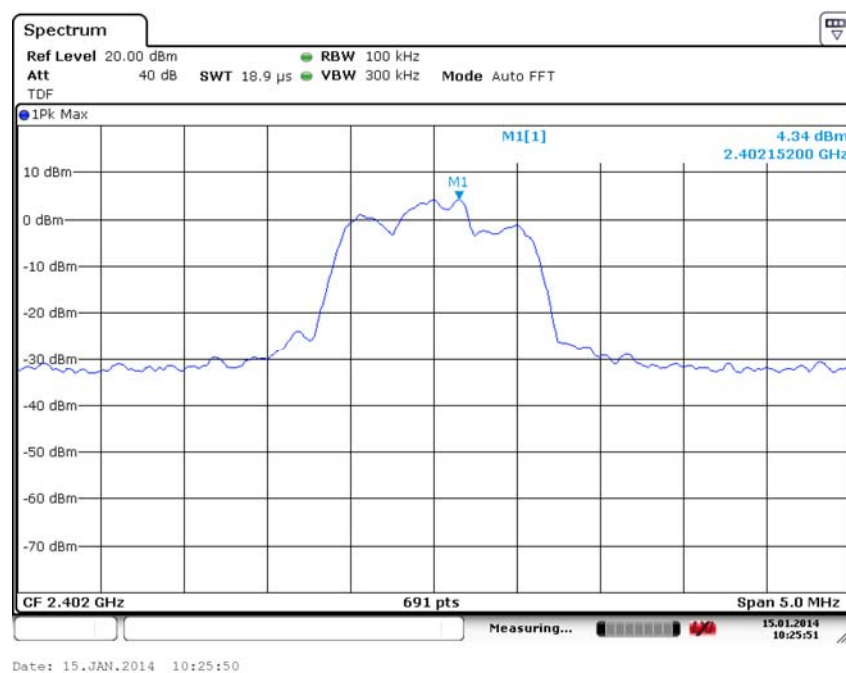
Fig. 31 Conducted Spurious Emission (8DPSK, Ch0, 2.402GHz)
