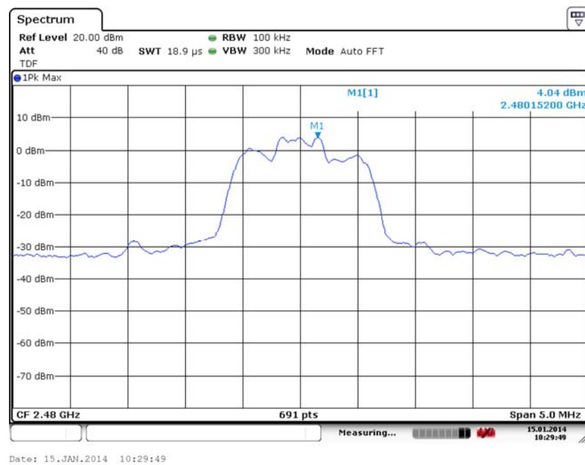
Fig. 37 Conducted Spurious Emission (8DPSK, Ch78, 2.480GHz)
