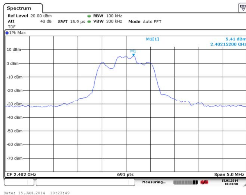
Fig. 22 Conducted Spurious Emission ( \pi/4 DQPSK, Ch0, 2.402GHz)
