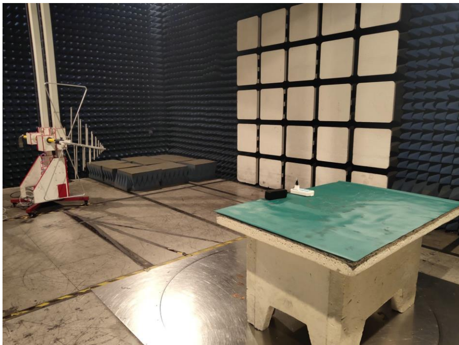
Photograph 2: Set-up for Radiated Spurious Emission, Up to 1GHz
