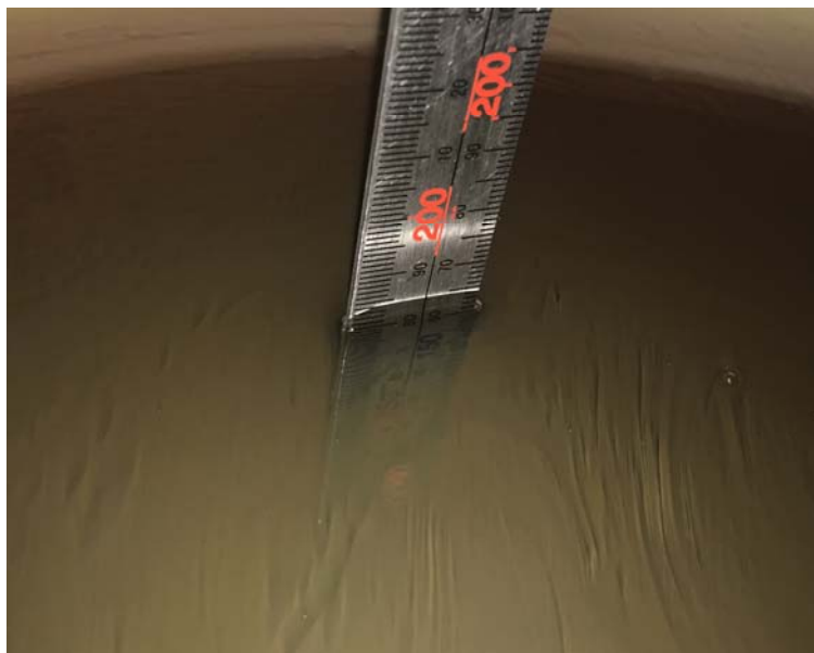
Liquid depth for SAR Measurement
