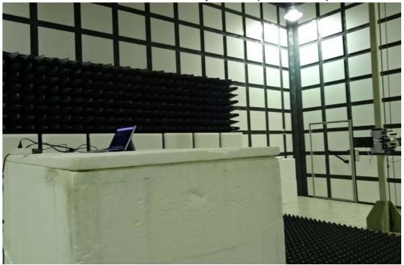
Radiated Emission Set up Photos (Front View)
