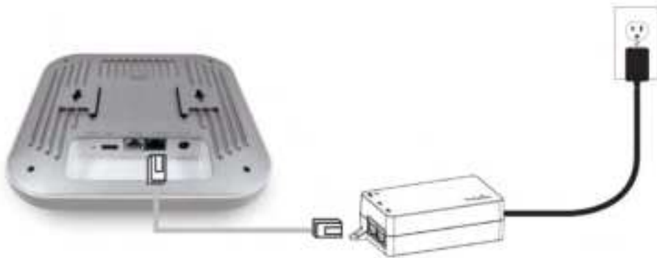
Access Point connected to PoE+ injector
