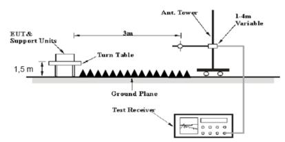
The radiated emissions were performed in the 5 meters distance, using the setup accordance with the ANSI C63.10-2013. The specification used was the FCC 15.209, and FCC 15.247 limits.
