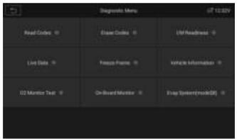
Figure 4-9 Sample OBDII Diagnostic Menu
