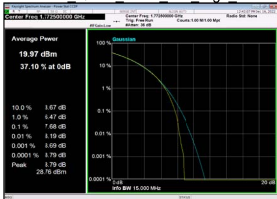
N66(15M)_CP- OFDM QPSK Outer Full High CH
