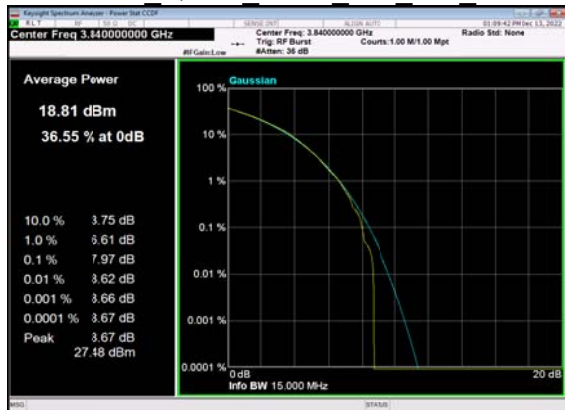
N77(15M)_CP-OFDM QPSK Outer Full Mid CH
