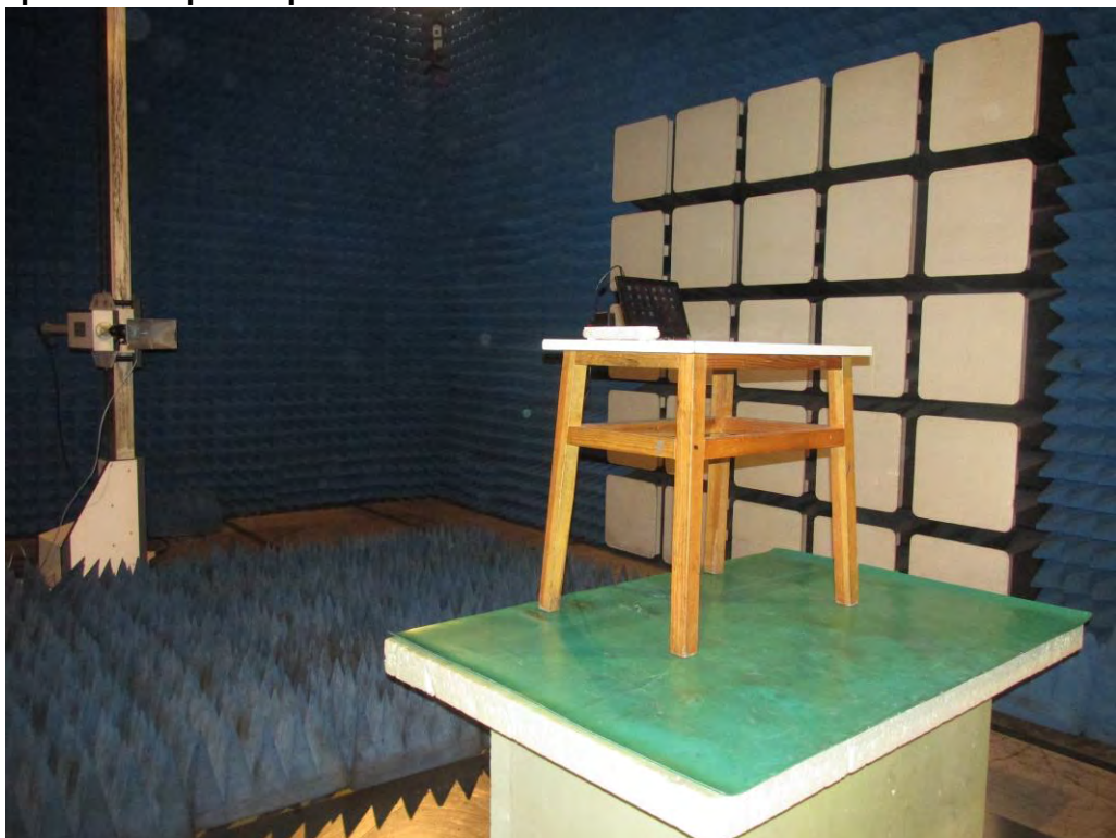
Photograph 4: Set-up for Spurious Emissions for 1 - 18GHz
