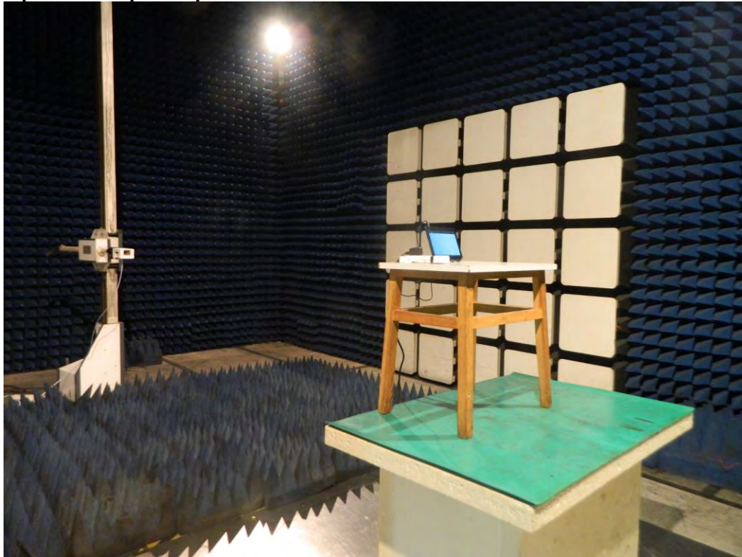
Photograph 5: Set-up for Spurious Emissions for 18 - 26.5GHz
