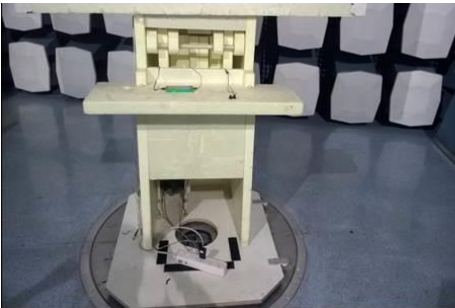
Picture 1. FCC Part 15C Radiated emissions
