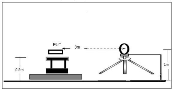
(B) Radiated Emission Test-Up Frequency 30MHz~1GHz
