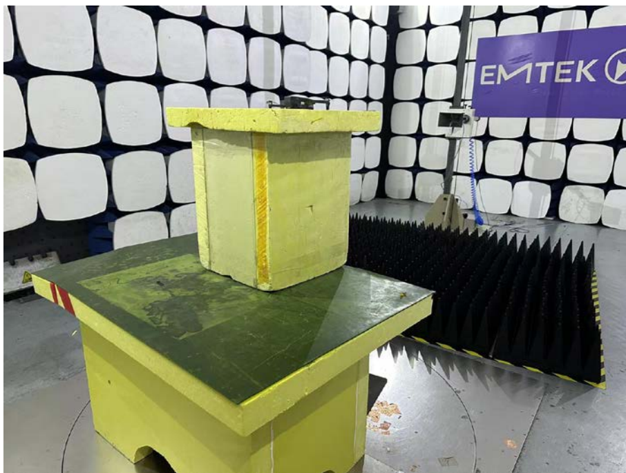
Spurious Emission Test Setup (Above 1GHz)
