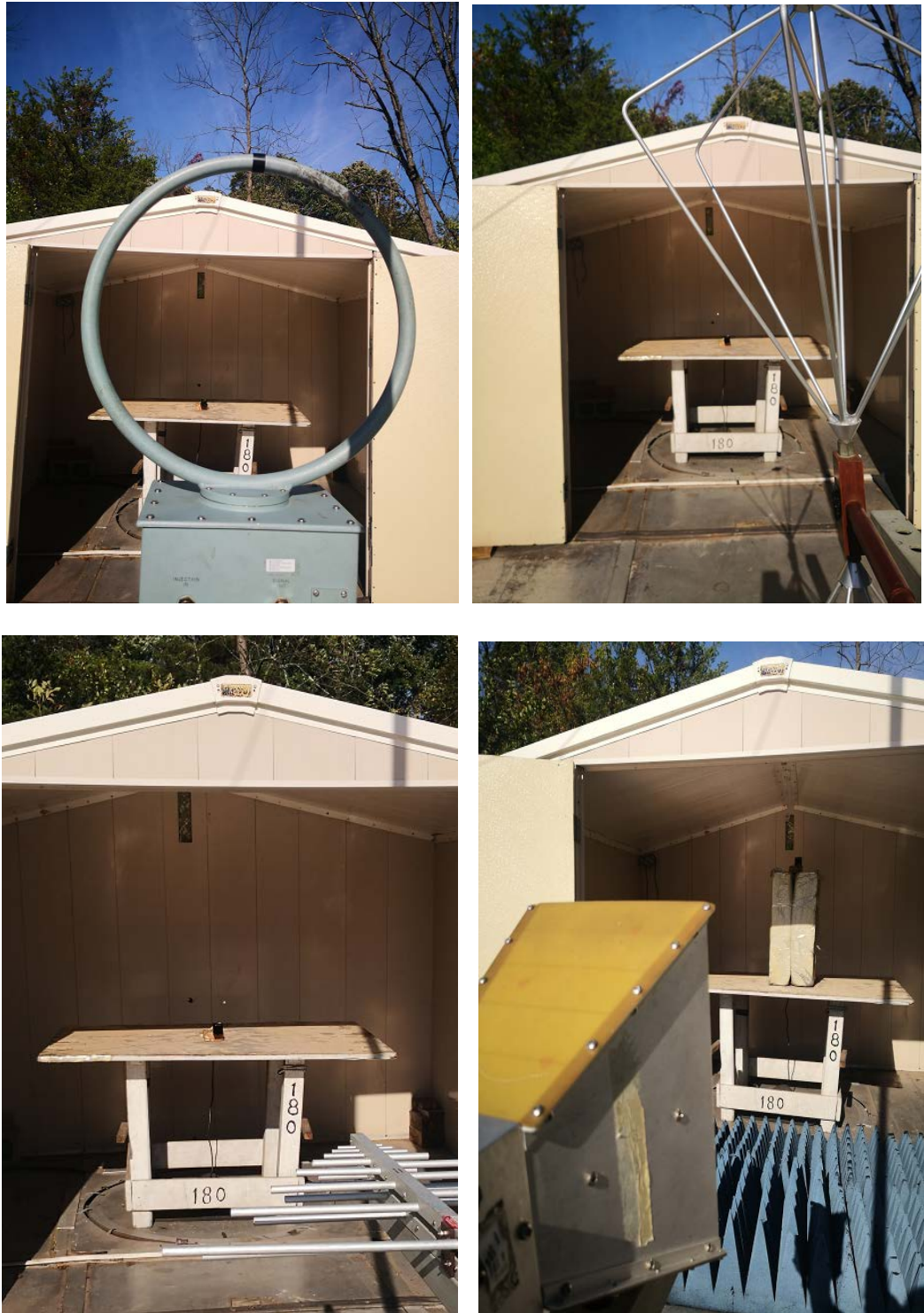
Figure 3.1 Radiated Test Setup
