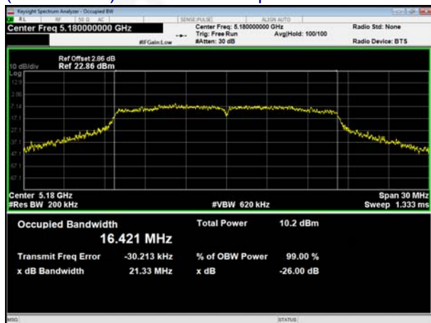
(802.11ac20) 99% Bandwidth plot on channel 36
