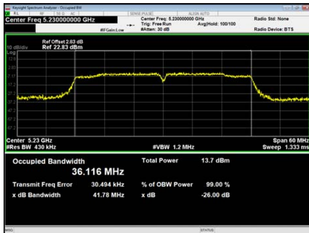
(802.11 n40) 26dB Bandwidth plot on channel 46
