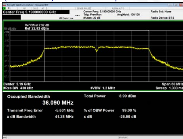
(802.11 ac40) 99% Bandwidth plot on channel 38
