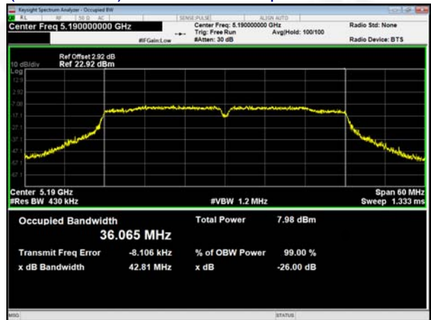
(802.11 ac40) 26dB Bandwidth plot on channel 38
