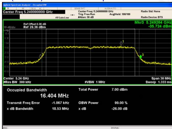
(802.11a) 26dB Bandwidth plot on channel 48
