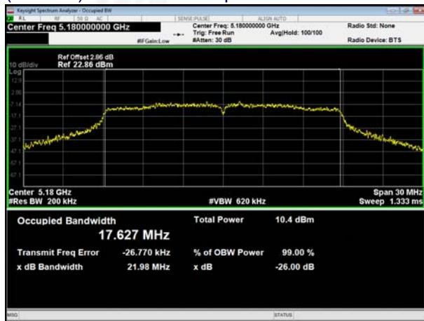
(802.11a) 99% Bandwidth plot on channel 36
