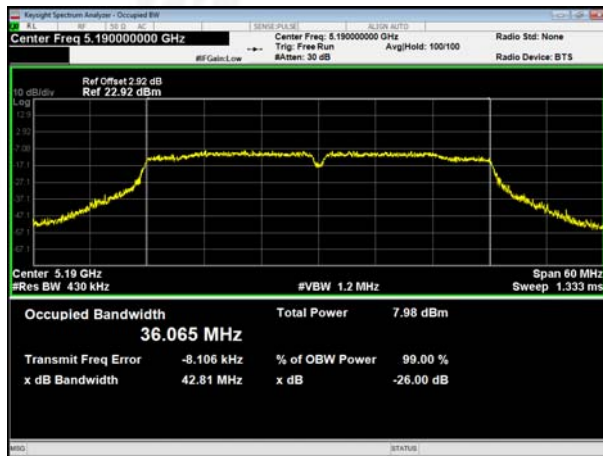
(802.11 n40) 26dB Bandwidth plot on channel 38
