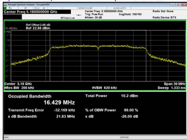
(802.11 n20) 99% Bandwidth plot on channel 36
