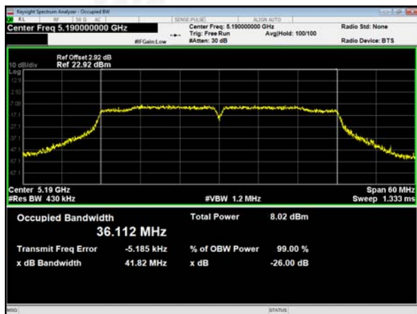
(802.11 n40) 99% Bandwidth plot on channel 46
