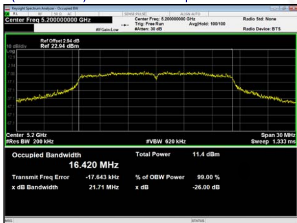
(802.11ac20) 99% Bandwidth plot on channel 40
