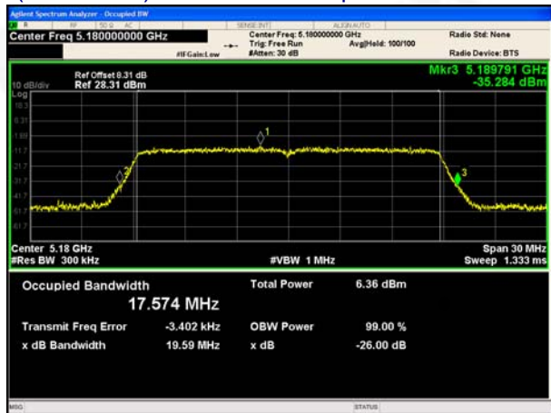
(802.11 n20) 26dB Bandwidth plot on channel 36
