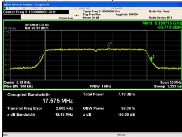
(802.11ac20) 26dB Bandwidth plot on channel 36
