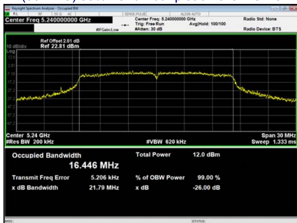
(802.11a) 99% Bandwidth plot on channel 48
