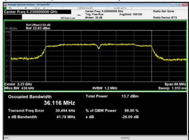
(802.11 ac40) 26dB Bandwidth plot on channel 46
