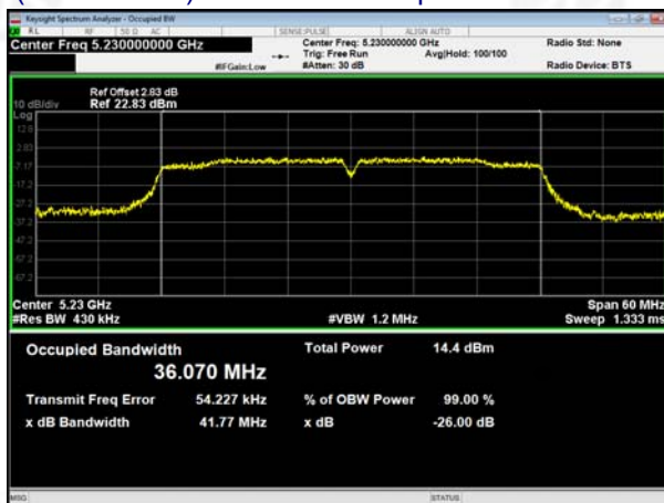
(802.11 ac40) 99% Bandwidth plot on channel 46
