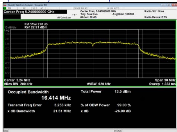
(802.11 n20) 99% Bandwidth plot on channel 48
