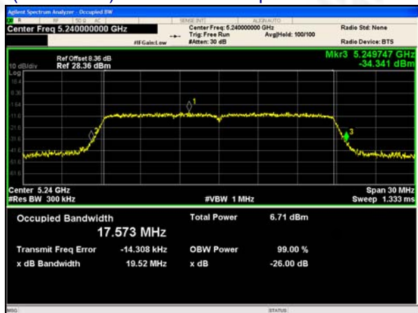
(802.11 n20) 26dB Bandwidth plot on channel 48
