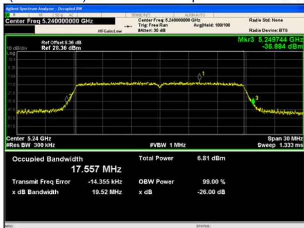
(802.11ac20) 26dB Bandwidth plot on channel 48
