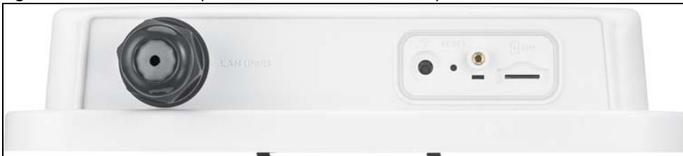
Figure 3 Bottom Panel (LTE7461-M602 / LTE7480-S905)
